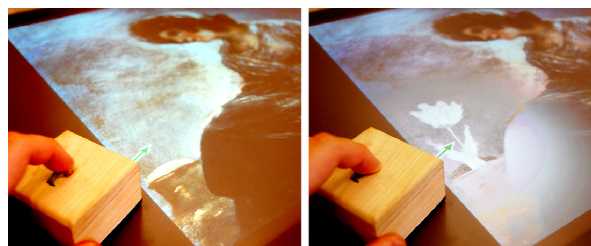
Figure 6. The puck reveals hidden content in a particular area of the painting by raising the rod (left). By pressing on it the x-ray layer can be revealed (right)
