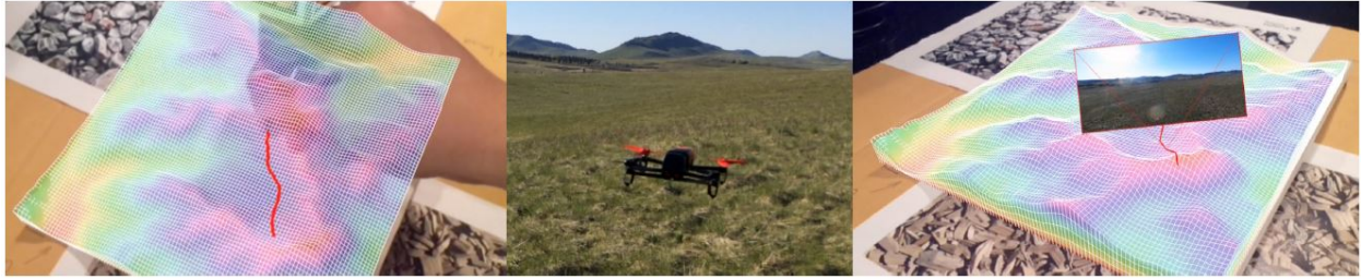
Figure 8: Illustration of the concept: Flying Frustum allows users to teleoperate an UAV with sketch-based gestures on a physical terrain model and streams the UAV's view frustum
