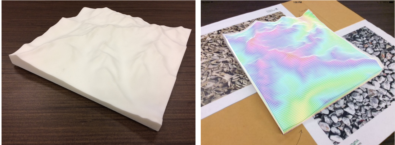
(a) Using a 3D printout model as a physical representation to the topographical terrain (b) Augmented reality visualization is superimposed onto the model
