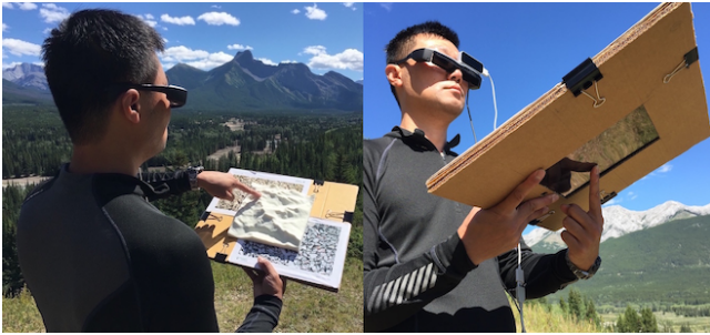
Figure 6: Using the front irregular topography surface to create spatial data by sketching (left); there is a back-of-device flat surface for interacting with the exiting spatial data (right).
