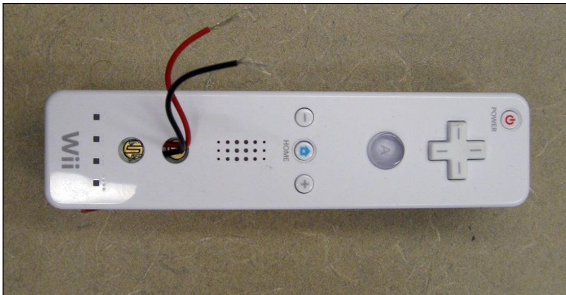
Figure 5.14 – A hacked Wiimote, with wires leading to the missing ‘2’ buttons
