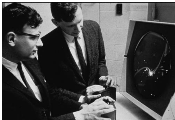
Figure 2.3 – Two men playing Spacewar! using custom control boxes
