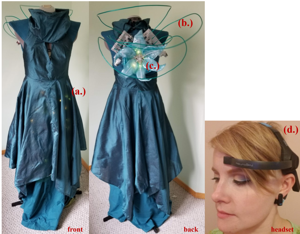
Figure 8 Automata on a dress-form mannequin. (a) the front of the dress with LEDs diffusing under the skirt, (b) the “wigglers” attached to a cam arm system, (c) a flower that opens and closes at fixed intervals, and (d) Kath wearing the EEG brain activity sensor. 25
