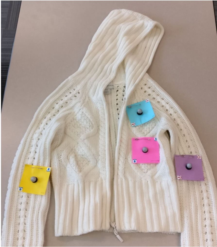
Figure 21 Tags attached to an existing garment before being detected by the mirror. The colored tags are attached using safety pins. A designer can quickly reposition the tags without rewiring the components or reprogramming the garment.
