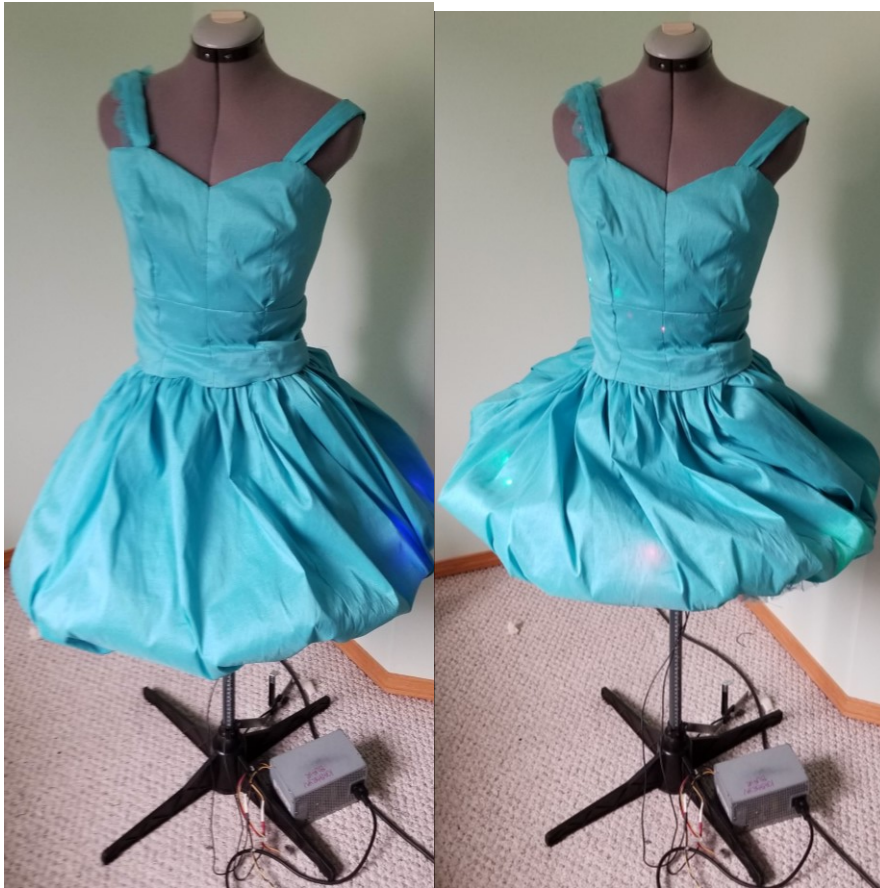
Figure 9 Positive Feedback on a dress-form mannequin. (Left) the dress in a low social media activity popularity, the skirt is lowered. (Right) the dress in a high social media popularity state, the skirt is raised. 27
