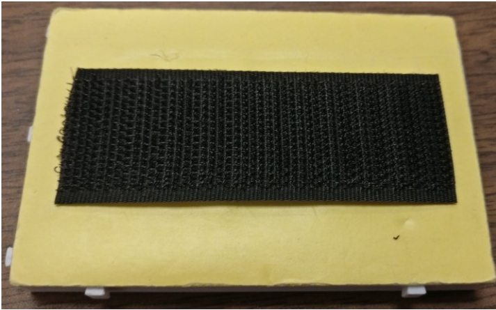
Figure 17 The bottom of an empty badge which includes a velcro piece for attachment.
