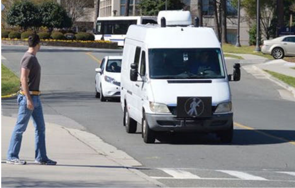
Figure 4: Interface display showing the symbol "don't cross" (Source: Clamann, Aubert, and Cummings [10]).
