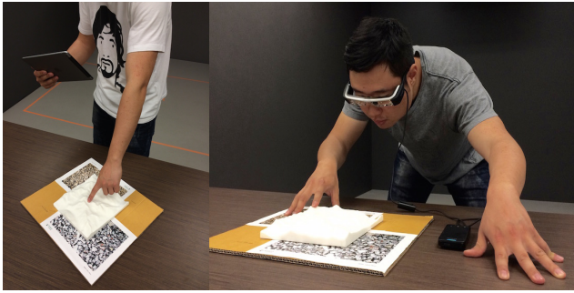
Figure 3: Flying Frustum's augmented reality devices including (left) handheld screen and (right) see-through headset
