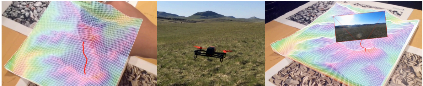
Figure 1: Flying Frustum ; (left) the operator draws a path using a pen on the augmented 3D printout of the terrain; (middle) the UAV, a quadrotor in the current prototype, flies along the path in the field; (right) live video footage streaming from the UAV is displayed as a view frustum situated at the correct location on the 3D printout, using augmented reality.
