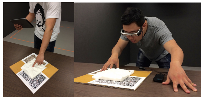
Figure 3: Flying Frustum 's augmented reality devices including (left) handheld screen and (right) see-through headset
