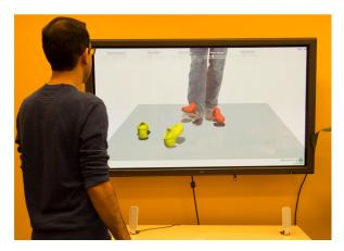
Figure 2. HappyFeet represents the feet of both local dancer (in yellow) and remote dancer (in red). This is superimposed on a video of the remote dancer, or instructional video.
