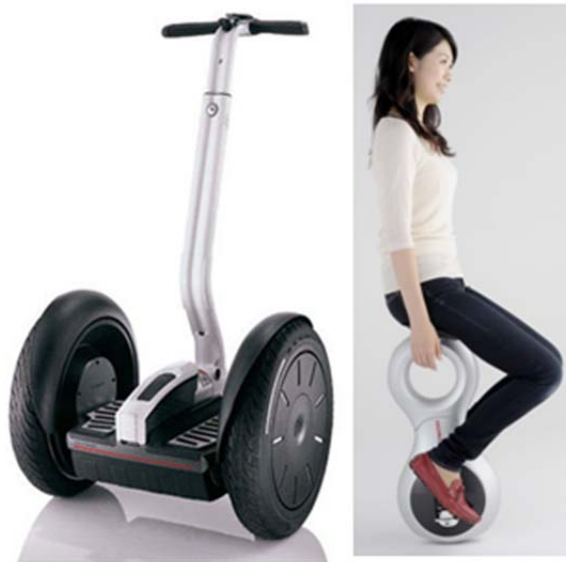
Figure 17 - The Segway (left, (Segway Inc.)) and Honda UX-3 (right, (Honda Motor Company Limited)) personal transporter devices. Both vehicles utilize an "inverted pendulum" style of locomotion
