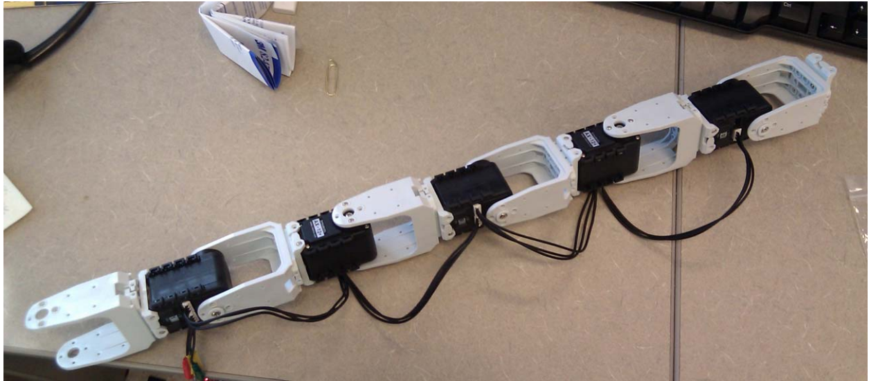
Figure 35 – Our motors proved too weak to form a sufficiently large chain for the Jungle Snake prototype’s body
