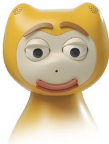
Figure 8 - The Philips "iCat" robot head. Resembling a cartoon cat, the iCat's facial features can change to express various emotions. (Philips Electronics)
