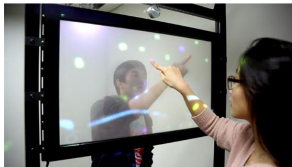
Figure 2.4: TransWall, a projection-based transparent display. The content on both sides was the same. (Heo et al. 2013)
