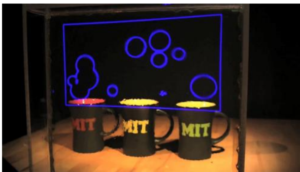
Figure 2.5: A transparent display that selectively scattered light at a particular wavelength (Hsu et al. 2014)
