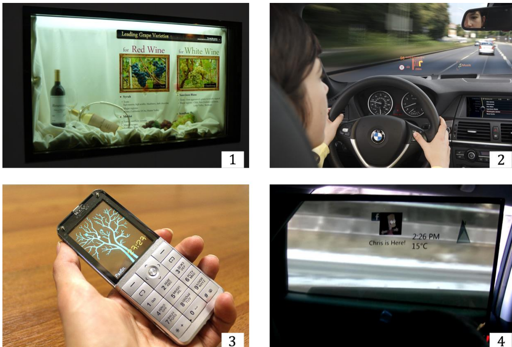
Figure 1.2: (1) a transparent display showcase (Humphries, 2010) (2) a transparent display integrated into the car windshield (Lysikatos, 2012) (3) a mobile phone using a transparent display as its screen (phoneArena.com, 2014) (4) a transparent display providing augmented reality information to the passenger in a vehicle (Li et al, 2013).
