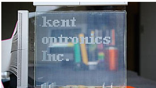
Figure 2.2: A monochromatic transparent display based on liquid crystal (Kent Optronics, 2014)
