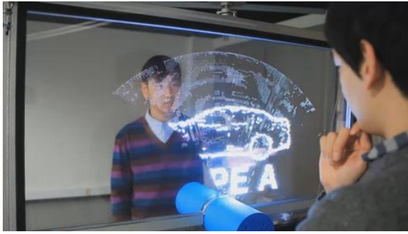
Figure 2.3: JANUS, a two-sided emissive transparent display making use of POV effect (Lee et al., 2014).
