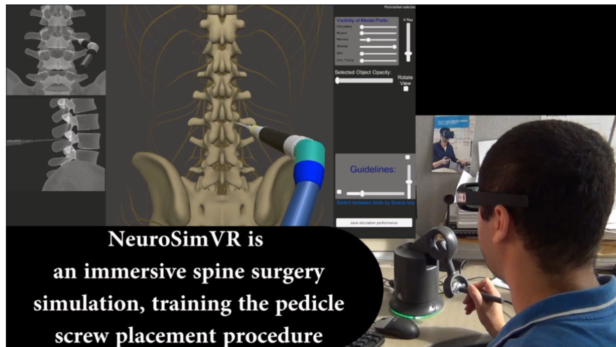
Figure 4.3: The interface of NeuroSimVR Simulator: X-ray views (left), perspective 3D view (center), and GUI controls (right).
