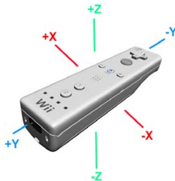
Figure 4.4 – The coordinate system of Wiimote
