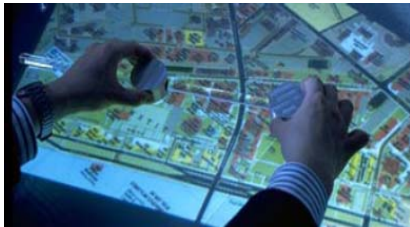
Figure 2.5 – Scaling device for zoom in/out on a digital map (Ishii and Ullmer, 1997)
