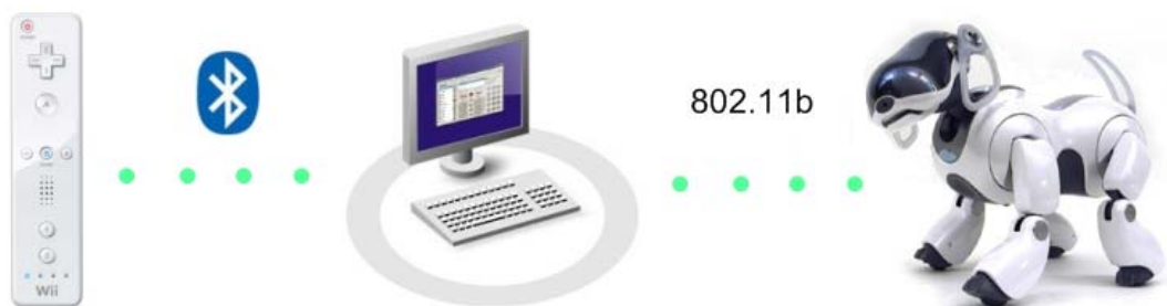
Figure 4.2 – Communicating between the Wiimote and AIBO through a PC
