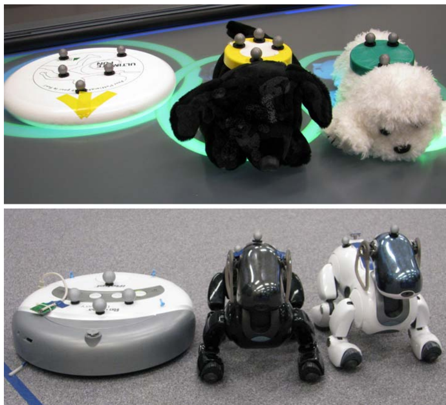
Figure 5.2 - Our tangible user interfaces and corresponding robots
