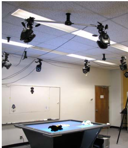
(a) The tabletop workspace with TUIs on top and the Vicon ceiling setup.
