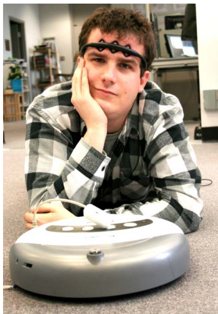
Figure 3.1: Our NIA-Roomba brain-robot interface prototype
