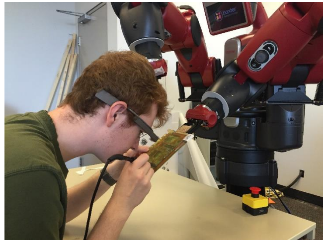
Figure 1. A user controls a robot to help them solder, seeing the perspective from the robot’s hand camera in Google Glass.
