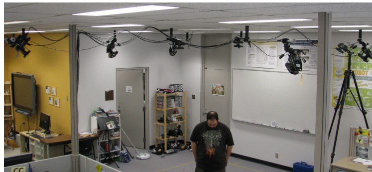
(b) ceiling-mounted vicon cameras
