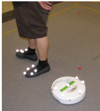
(c) reflective markers on person's slippers and the robot (markers artificially highlighted by camera flash)
