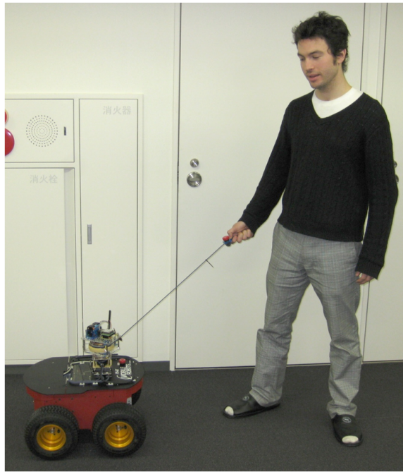
Figure 1.1: our dog leash interface for leading a robot
