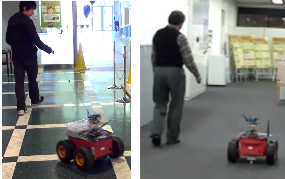
(a) robot directly behind the person (b) robot behind and to the side of the person
