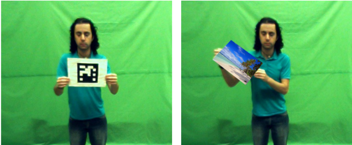
Figure 5.15 The fiducial marker is hidden by the image an augmented reality version of the postcard image.
