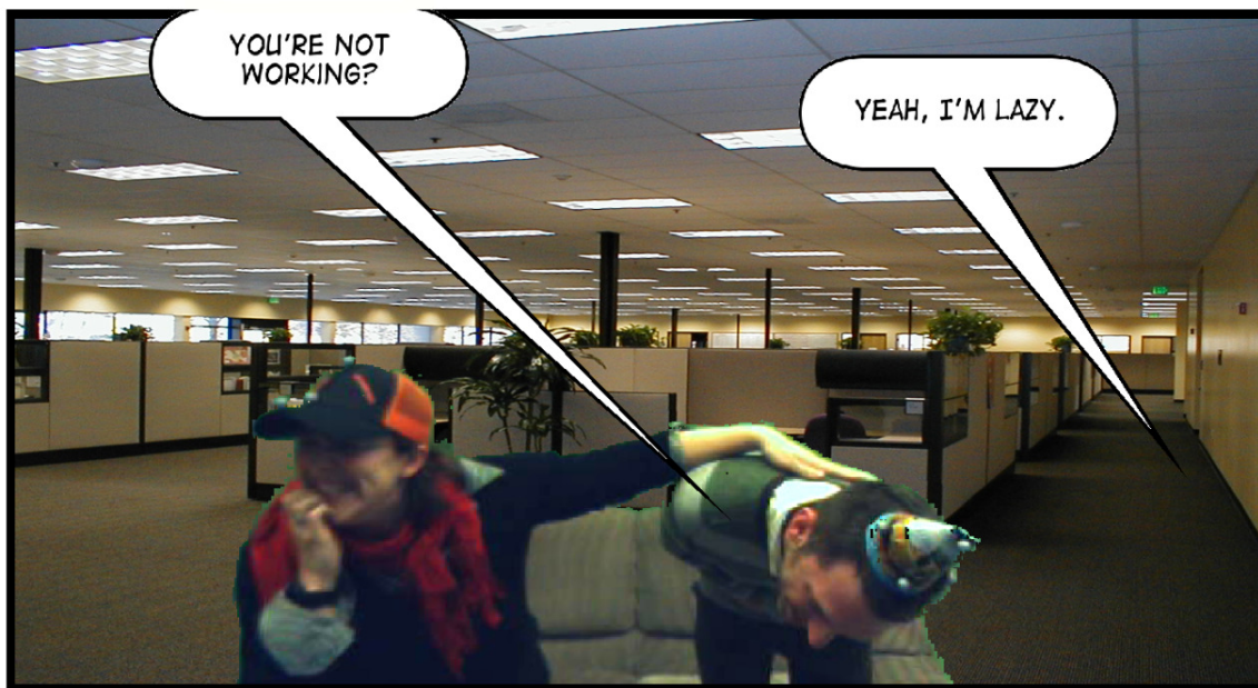
Figure 5.27 The speech bubble arrows don't appear correctly when the tracking system is affected by noise.
