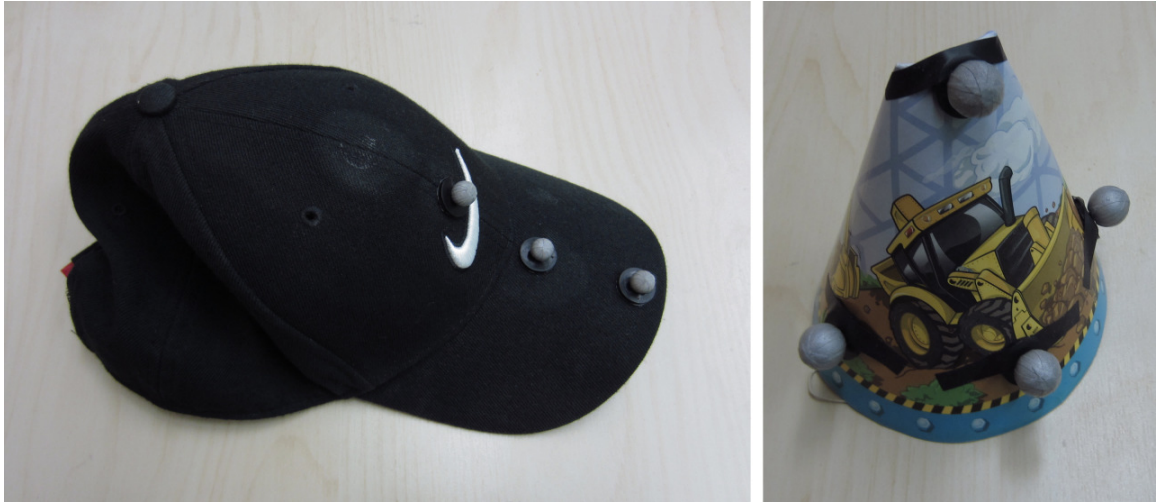
Figure 5.19 The hats used for tracking have a different number of markers in unique patterns.
