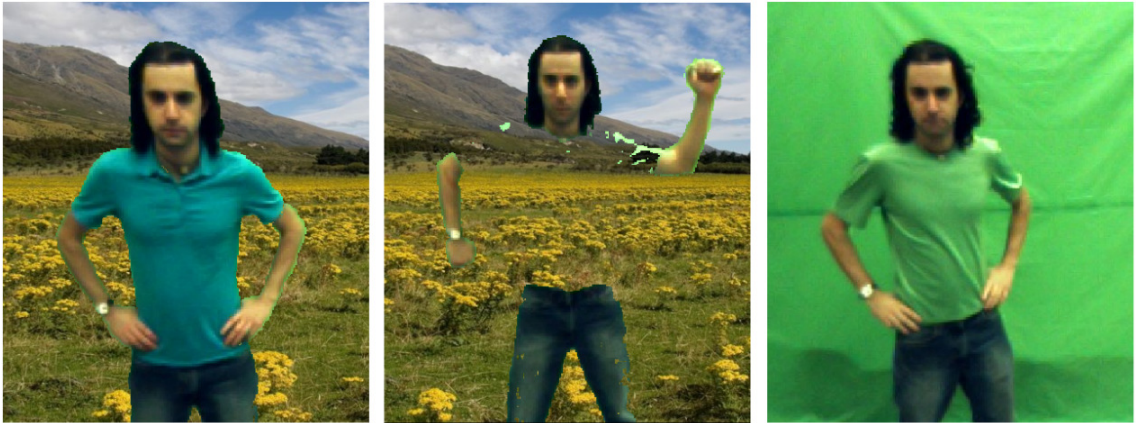
Figure 5.7 Two examples of the chroma-key filter. The subject in the middle image is wearing a green shirt. The right image is the original image.
