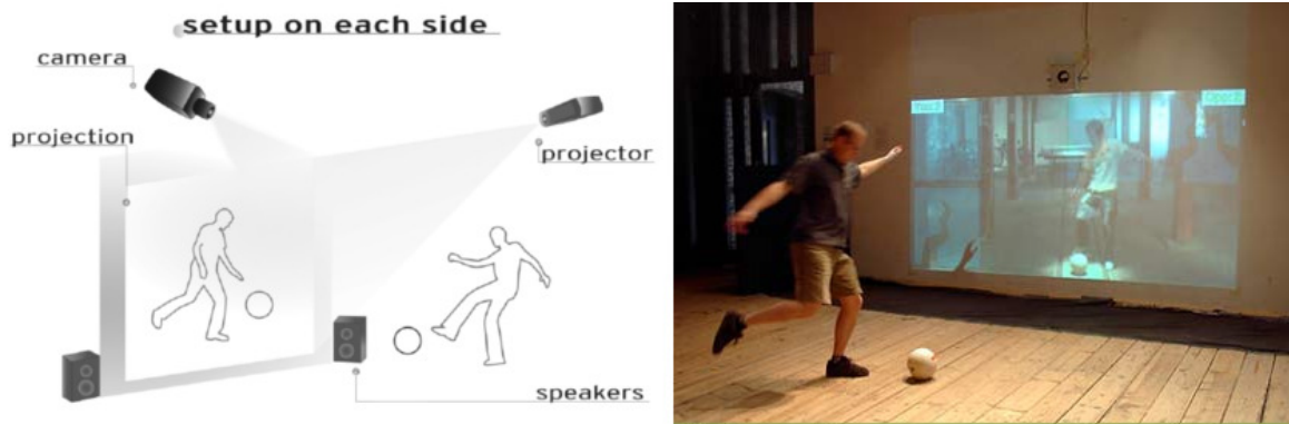
Figure 2.10 Breakout for Two uses a camera and projector to connect two remote players (Mueller).
