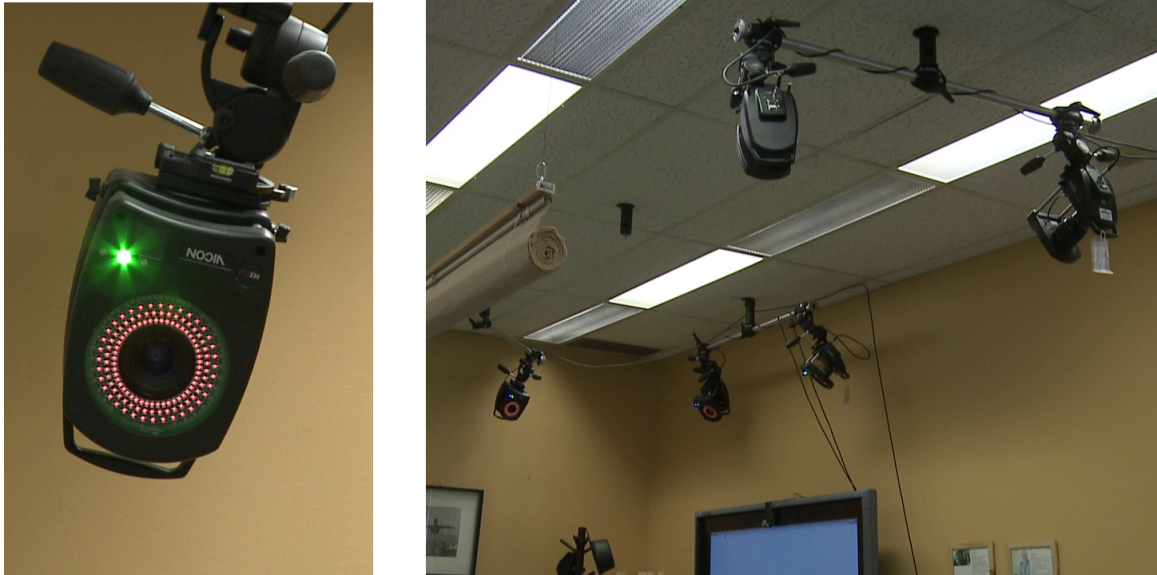
Figure 5.17 Individual Vicon camera and arrangement of cameras mounted on the ceiling around the game space.
