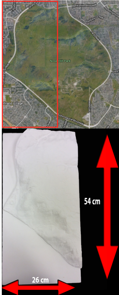
Figure 7.2: (top) Google map image of the wilderness park near our university. The red rectangle is the area which we 3D printed and (bottom) the 3D printout of the area marked in the google map image.
