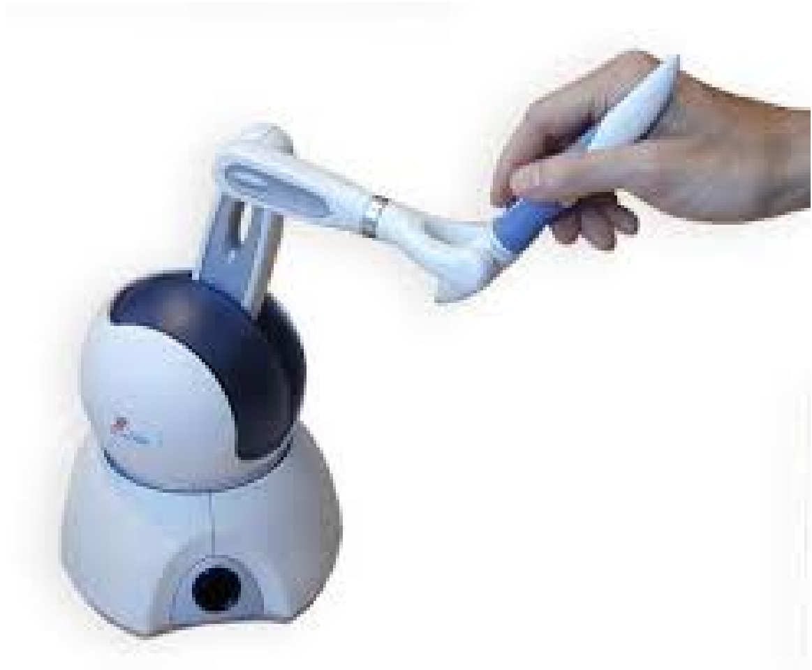
Figure 7.7: The Phantom Haptic Interface. The stylus could also be used on 3D physical maps for various operations such as sketching, annotating, and erasing.
