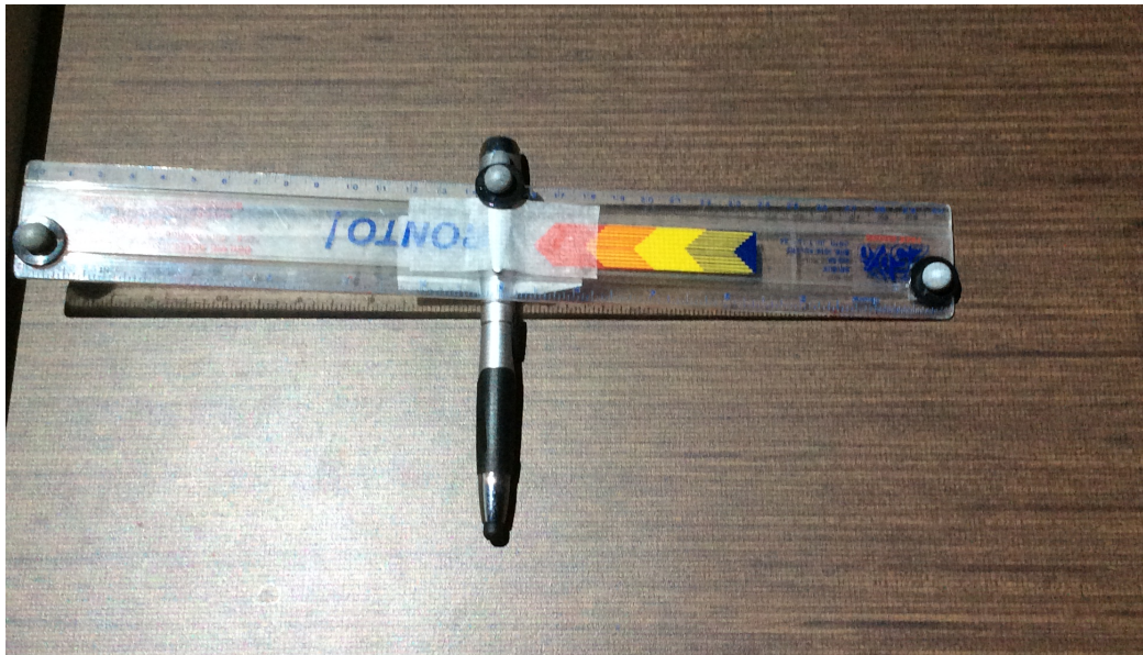
Figure 7.6: Our Stylus prototype with 3 vicon markers. The stylus has been elongated by attaching a scale, for better visibility of the markers.
