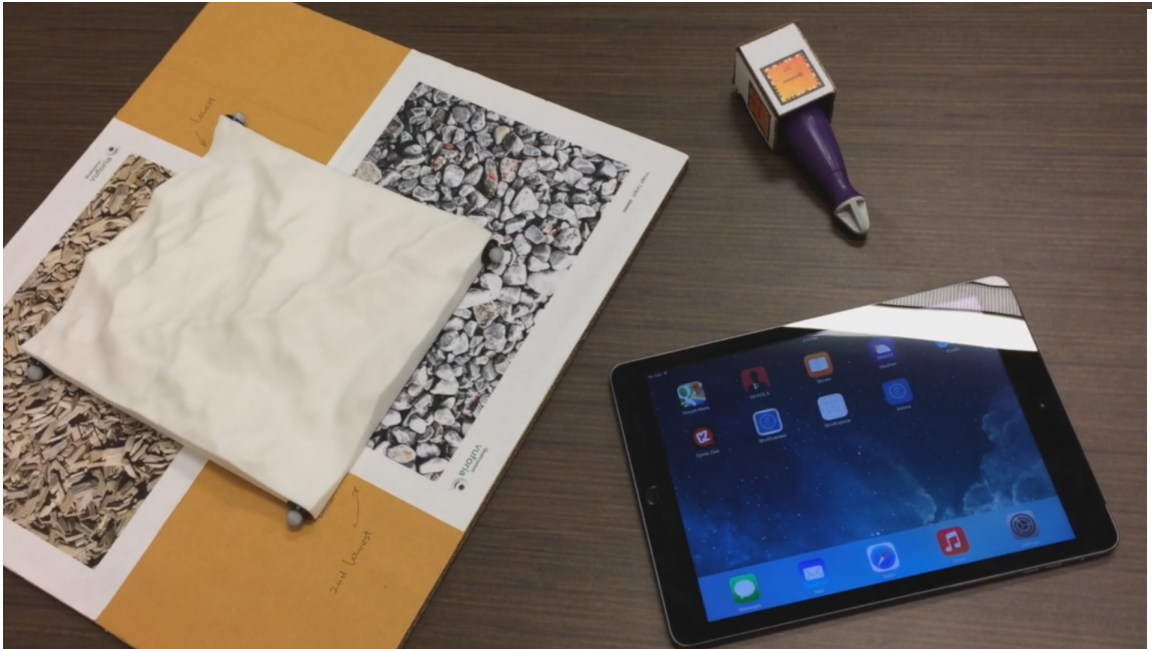
Figure 4.5: The overseer interface which consists of the 3D printout of the terrain, an iPad as the AR device and a stylus.
