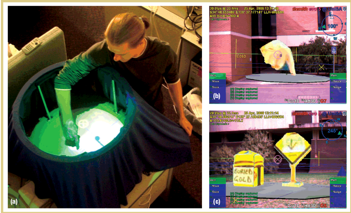
Figure 2.9: God-Like Interactions by [Stafford et al., 2006]. (a) indoor user pointing at a location on the table-top surface, which contains the representation of the outdoor world. (b) Outdoor AR view showing the indoor user’s hand appearing form the sky and pointing toward a location in the distance.(c) Physical objects used as props to convey extra meaningful information about the environment.
