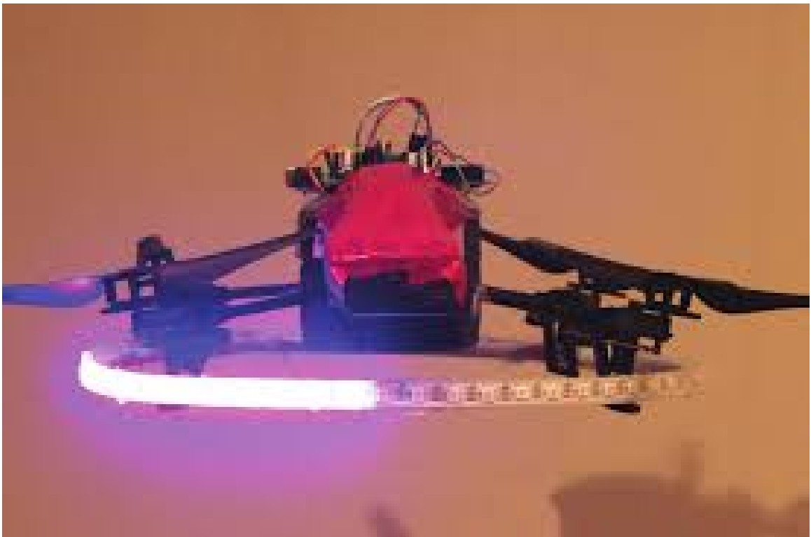
Figure 2.17: [szafer et al.2015] explored the design of visual signalling mechanisms for flying robots to support the expression of robot intent and increase usability in collocated interactions.
