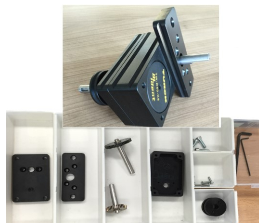
Figure 4. Gearbox object (top) and its discrete parts (bottom)
