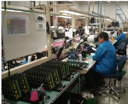
Figure 42: A possible workspace of Baxter at the DSM assembly line - the robot would inspect the boards on the left, close to the workers testing the functionality of the components.
