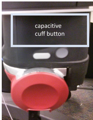
Figure 3: The capacitive cuff buttons enabling the zero-G mode
