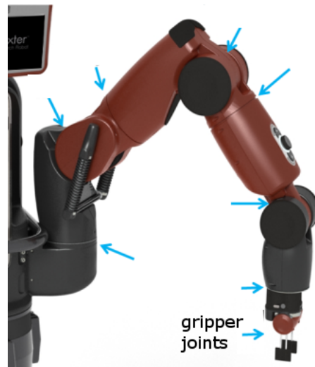
Figure 7: The different joint types in the kinematic chain, all joints are marked by an arrow. Only the gripper joints are prismatic.
