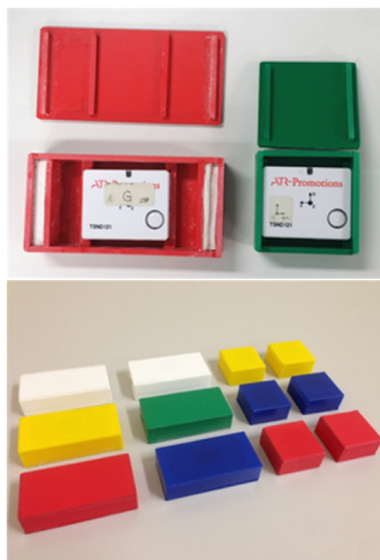
Figure 2. Prototypes of the Bluetooth-IMU-sensor embedded blocks for the preliminary study.
