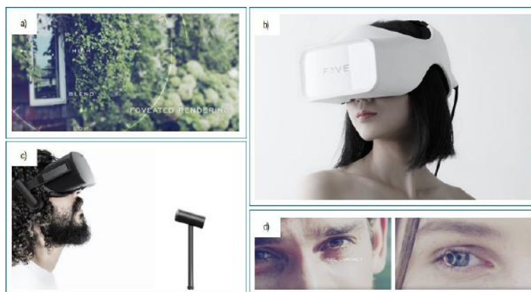
Figure 9: Oculus Rift [28] uses sensor fusion and Constellation tracking to provide head-tracking input – (c). FOVE [29] uses infrared sensors for eye tracking – (a, b, d). By using eye-tracking, the FOVE system allows two innovative features: eye contact monitoring and foveated rendering. Foveated rendering refers to loading high-resolution textures where users are actually looking, and optimizing out-of-focus areas with lower-resolution or fewer effects.
