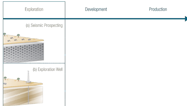
Figure 22: Seismic studies and exploration wells are some of the efforts performed in the exploration stage.
