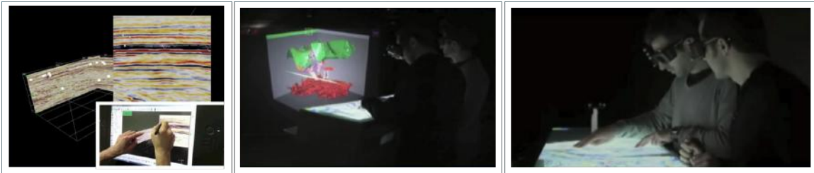
Figure 58: On the left, SeisTablet integrates a shared monitor with tablets that support pen and touch interaction for seismic interpretation. On the middle and right, Slice Inspector combines a 2D multi-touch interface with a 3D large display for the analysis of seismic data.
