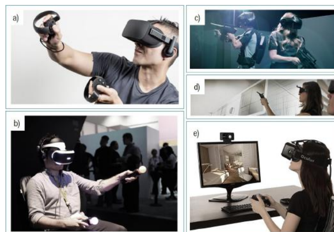
Figure 7: Examples of hand-held controllers. Oculus Touch [18], Sony PS3 Move [19], THE VOID Nova IV Gun [20], and WorldViz Wand [21] are tracked controllers – (a), (b), (c), and (d), respectively. MOGA Pro Controller [17] is a non-tracked gamepad – (e).
