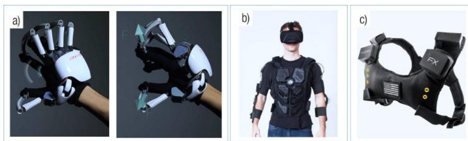
Figure 15: Dexmo (a) provides force feedback, while Null Space (b) and KOR-FX (c) suits simulate tactile feedback.
