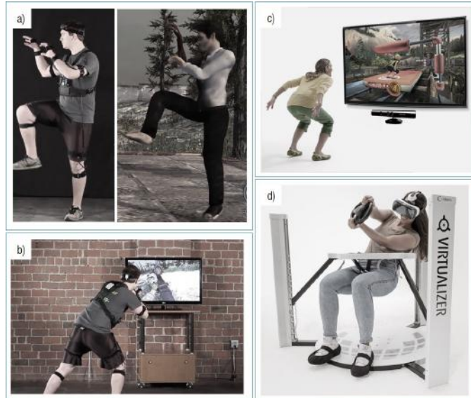
Figure 10: PriorVR suit [32] places inertial sensors onto the user's body, while Microsoft Kinect uses optical-based sensors placed on an add-on peripheral to provide full-body tracking input. – (a, b) and (c), respectively. Cyberith Virtualizer [30] is a treadmill that uses motion sensors in its base plate, pillars, and ring to provide foot tracking input – (d).
