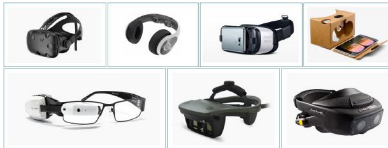
Figure 12: On the top row, HTC Vive [40], Samsung Gear VR [41], and Google Cardboard [42] are non-see-through HMDs. On the bottom row, Vuzix M100 [43] and NVisor ST50 [44] are OST HMDs, while Visette45 [45] is a VST HMD.
