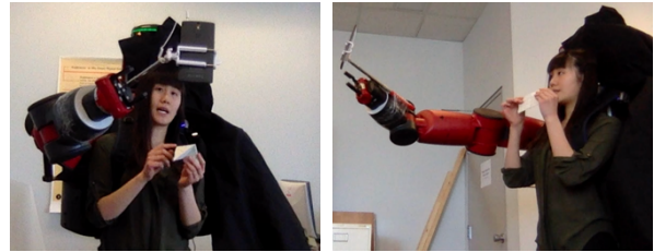
Figure 2: Selfie task with Baxter robot acting as SRAs.
